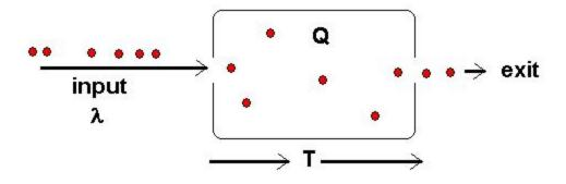
The mean values  $\overline{\lambda}$ ,  $\overline{Q}$ ,  $\overline{T}$ , are not independent. They are linked by Little's Theorem: (1961):
