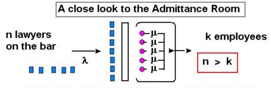
The written files enter the Admittance Room with rate λ according to a Poisson process. There are n emplyees with common service rate  $\mu$ . Both hypotesis are plausible and experimentally proven to be correct.
