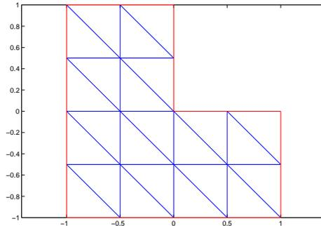
Figure 1: Initial mesh for the L-domain
