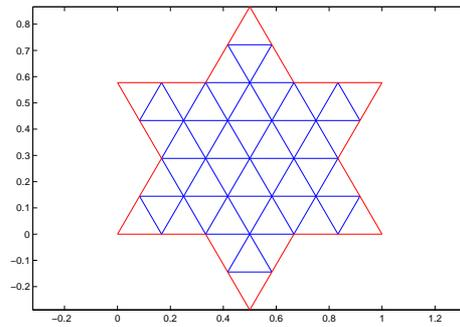
Figure 2: Initial mesh for level 1 approximation of the Koch domain
