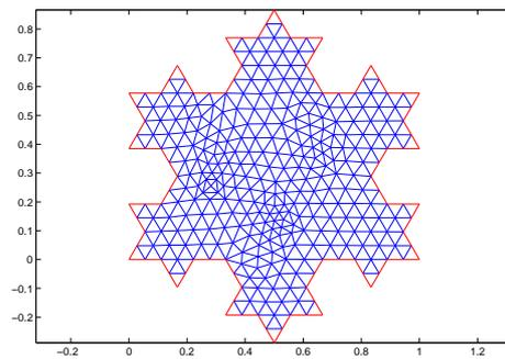
Figure 3: Initial mesh for level 2 approximation of the Koch domain
